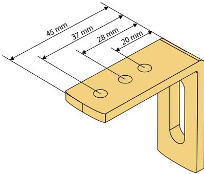
**Wall fixing bracket metal 50 mm**
