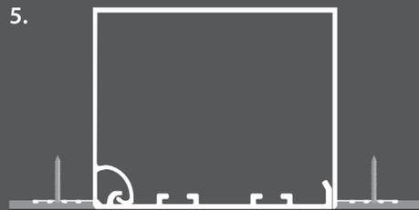
5. Closed covers can be used for the preparation of future options or they serve for an uniform optique on the ceiling.
