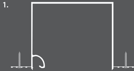
1. Blindspace®Boxes can be equipped during the dry construction mounting with a power cord.
