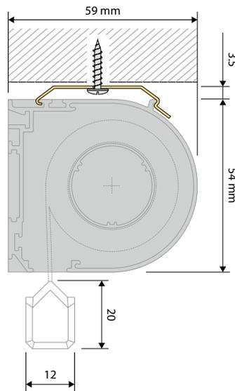
Window sash fixation with profile block holder
